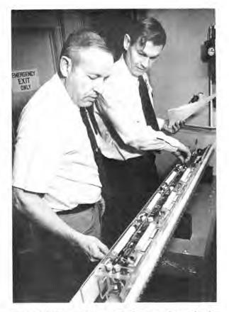
PROTOTYPE drilling head that employs shocks generated by electrical detonations was assembled from "off the shelf" components to prove feasibility of the concept. Gordon Harvey (5724) and Bob White (2315) check the unit.
